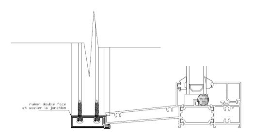
4. Seal the junction between the extension part and the original frame. Also apply the sealant at the corners of the extension.
