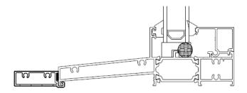
3. insert 2 # 8 screws at each extensions corner junction to connect the next frame side extensions to the other.
