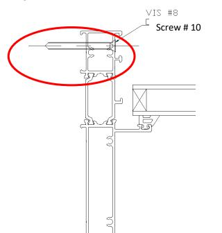
3. Install back the glazing molding that was removed by ensuring that it is clipped back as it was at first.
